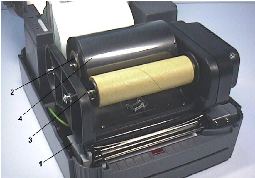
Placement of ribbon supply roll
