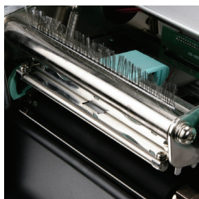
Easy to change, low-cost printhead assembly
